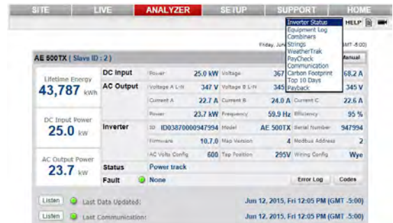
Fig 7 Check ANALYZER > Inverter Status to see data received from the inverter
