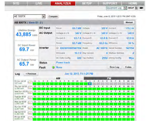
Fig 13 Log shows all inverter readings for last 30 days with record of fault messages for diagnosing problems
